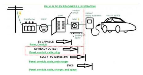
**EV Capable Space**: a vehicle space with electrical panel space and load capacity to support a branch circuit and necessary raceways, both underground and/or surface mounted, to support EV charging
